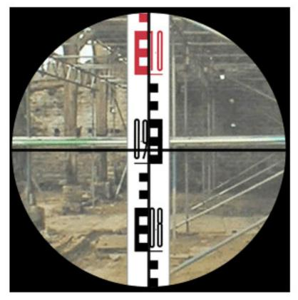
We align the theodolite view **horizontally**, then focus onto the staff.
