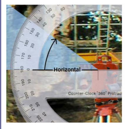
The angle between horizontal and the top of the building that the theodolite has measured is represented in the diagram above.
