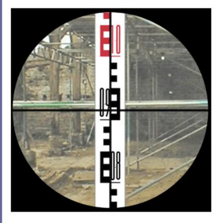
The reading of 0.915m we took from the staff is the distance from the ground to the bottom of the blue triangle.
