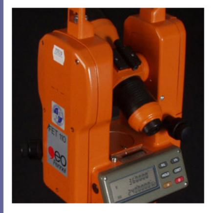
The theodolite display gives a digital readout of the angle between horizontal and the top of the building.
