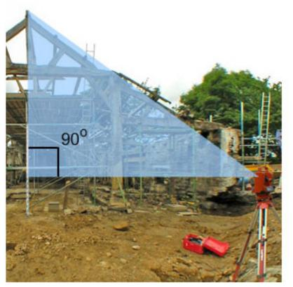
We know the theodolite was aligned **horizontally** to the ground when the staff reading was taken. We also know the staff is aligned **vertically** to the ground.
