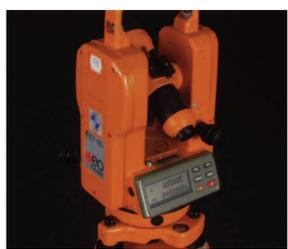
The theodolite display gives a digital readout of the angle between horizontal and the top of the building.
