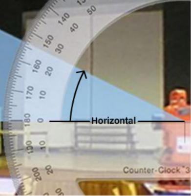
The angle between horizontal and the top of the wall that the theodolite has measured is represented in the diagram above.
