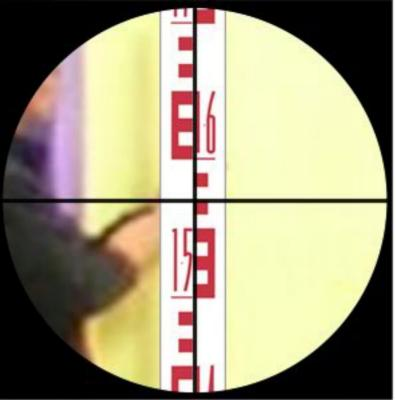
We align the theodolite view to **horizontal**, then focus onto the staff.
