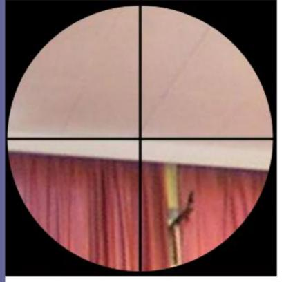
We then point the theodolite viewer at the top of the wall and align the crosshairs to it.
