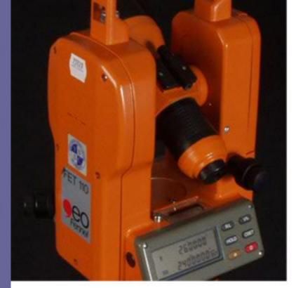
The theodolite display gives a digital readout of the angle between horizontal and the top of the wall.
