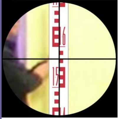
The reading of 1.57m we took from the staff is the distance from the ground to the bottom of the blue triangle.
